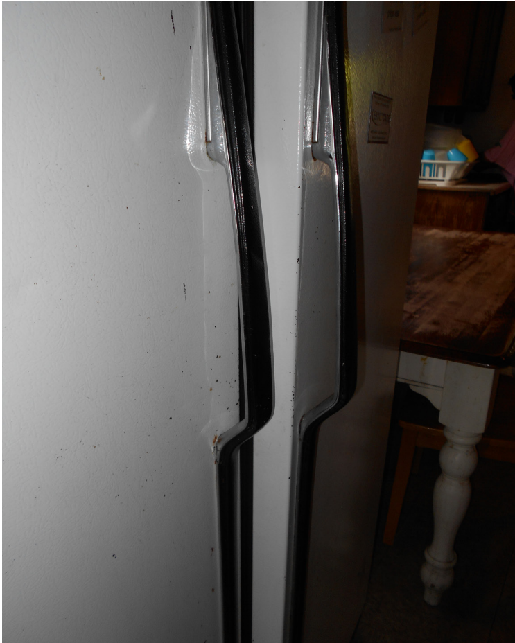
Photo 10 - Refrigerator did not latch-inside temperature was 48 degrees (fridge temp is suppose to be 40 degrees or under to ensure food does not spoil)
